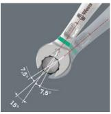
Thanks to the open end side offset by 7.5°, double hexagon geometry and an adjusted application method (placement - screwdriving - turning - replacement - screwdriving - turning, etc), even screwdriving challenges allowing a pivoting angle of less than 30° can be solved.
